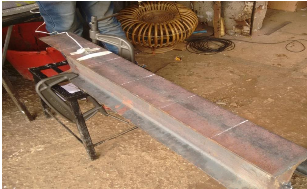
Fig 8: Experimental set up for strain measurement.
